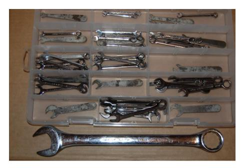
Unless you work on large machines, you probably won't need a 1" wrench as shown at the bottom. Ignition wrenches were originally made for working on automotive ignition systems, but are usefull when tightening small fasteners on a robot chassis or electronics panel.
