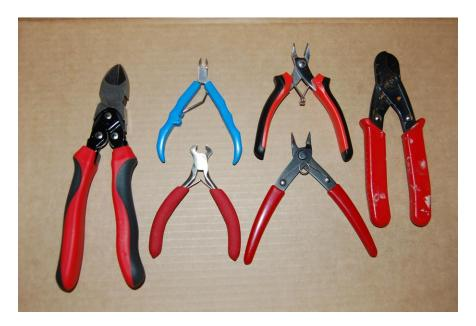
Wire cutters do just that. A variety of types are available. Diagonal cutters are needed. If you make circuit boards with through-hole components, a pair of flush cutters are need to trim the leads sticking through. Cable cutters (right) make clean cuts through larger materials like coaxial cable.
