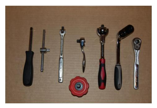
A variety of drive tools is useful, also. On the left is a spinner handle with a drive socket in the handle. It lets you turn sockets by hand, and the drive end lets you inset a sliding t-bar or breaker bar (next) to apply more torque. Tiny ratchets are needed for small places. Ratchets that let the head tilt or pivot are useful for hard-to-reach places.
