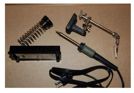
A soldering iron is need for some assembly. A stand holds it out of the way. A "helping hands holder" can hold the circuit board or components while you solder them. Some of the cheap models are not made well and can move around in use.
