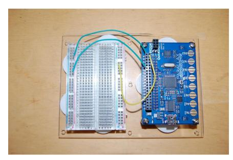
It can be used as a guide when cutting plexiglass with a special cutter to make board holders. Having both the microcontroller board and breadboard mounted together on a solid structure can make projects flow smoother, and have less problems with wires pulling out.
