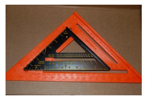
A speed square is useful when you are laying out project enclosures. Once the holes are layed out, you can use either a corded or cordless drill to drill them.
