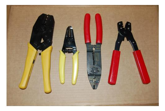
Wire stripping pliers (2) have notches for different sizes of wire, and let you remove the insulation without damaging the wire. Some crimping pliers are used for automotive type connecters (1,3), D-sub crimpers are used for D-sub connectors, telephone crimpers and Cat-5 crimpers are used for their connectors.
