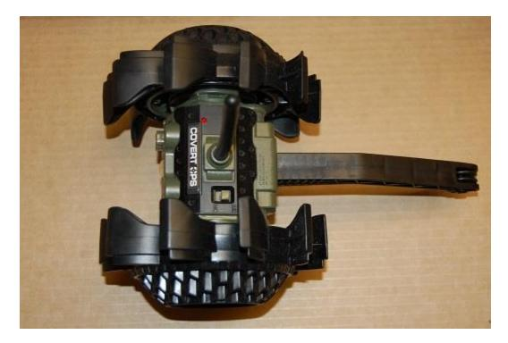
This skid steer only has two drive wheels. Due to lack of weight on the arm in the back, this vehicle has a tendency to rock forward when it stops. Since it only has two drive wheels, it can turn very quickly which makes the first person camera view blurry.
